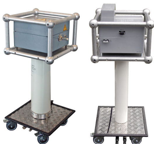
Figure 2: ICMflex (right) and T-filter (left) for 50 kV
