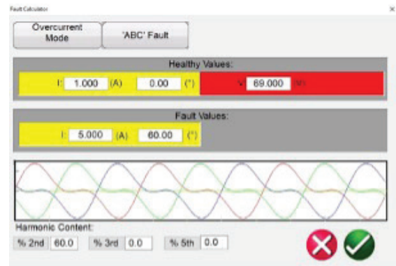
Figure 8: Fault Calculator – Overcurrent Mode with 2nd Harmonic content
