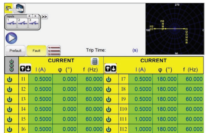
Figure 33: 12-Currents Simulating Bus Differential Scheme
